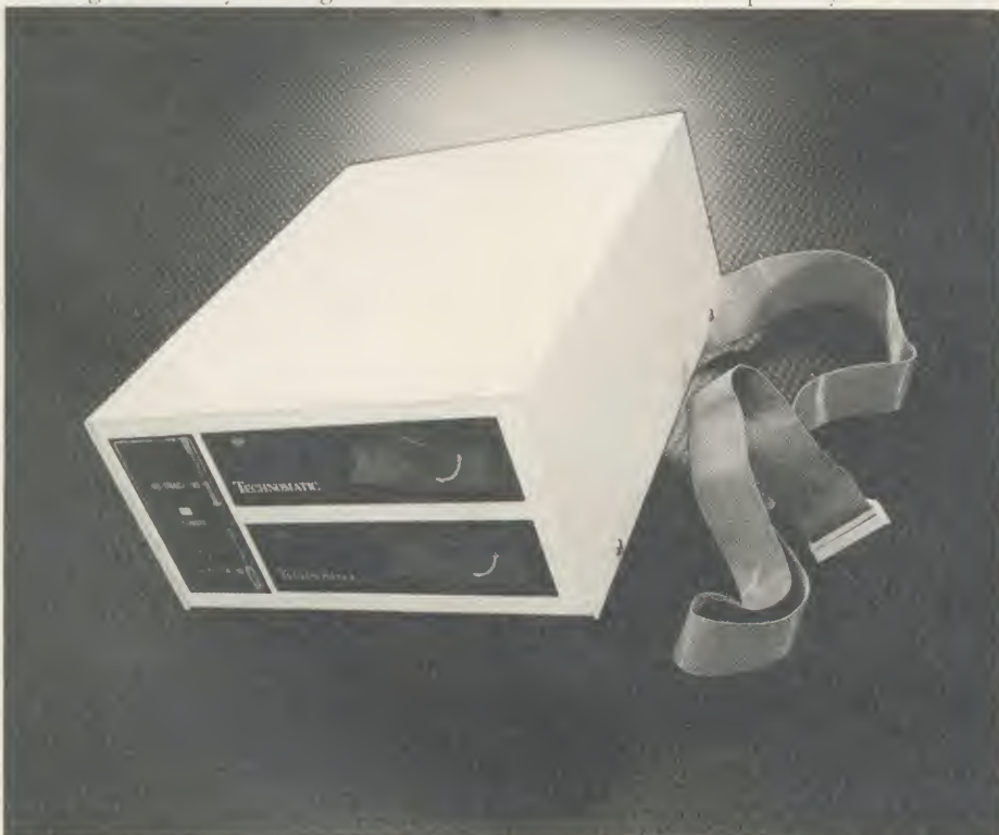
Technomatic's stacked dual 40/80 track switchable drives: the company offers a wide and varied range of drives
